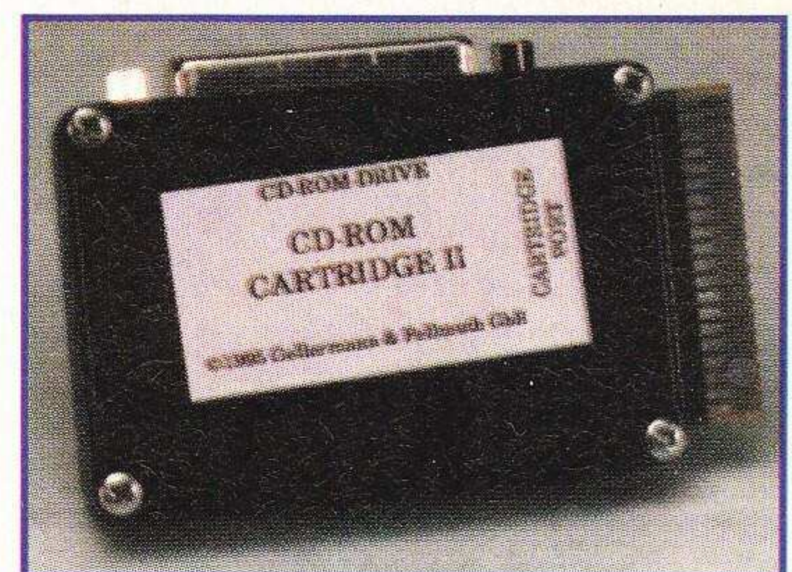
This small box connects the IDE CD-ROM drive to your ST's cartridge port.
